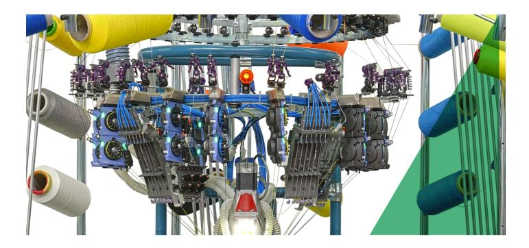
Single-cylinder INTARSIA electronic knitting machine with 4 reciprocating feeds and 2 selection points (3 technical ways) per feed and per rotating sense, for the production of intarsia products with cushioning areas knitted in sculpted terry.
